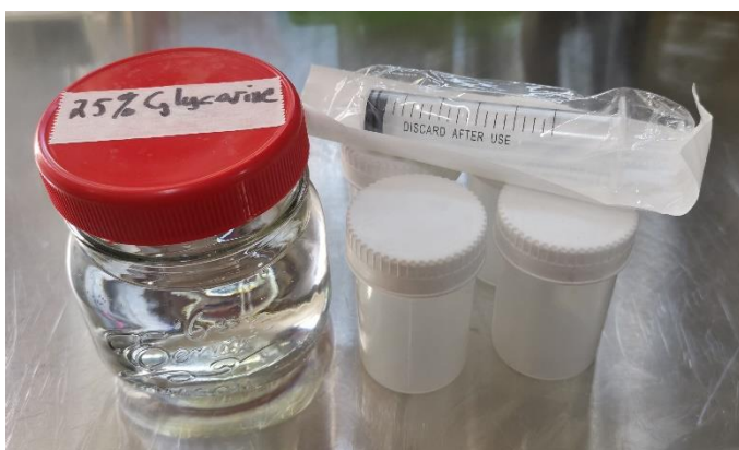
Figure 4. Materials required to prepare frozen yeast cultures. Including a short, 200ml Mason jar with a microwavable lid, 40ml specimen bottles, and a 10ml syringe.
